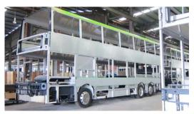
**LEFT:** Gemilang produces a wide range of bus bodies, including the double deck coach shown here. **RIGHT:** Early simulation allows to reduce costly physical testing on large bus structures.
